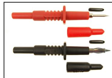
**TPR/1S** Spiked test probe. Unfused. Has 4mm. shrouded socket connection, so converts 4mm. shrouded plug into a test prod lead. 1KV CAT III with tip cover fitted, CAT II without.
